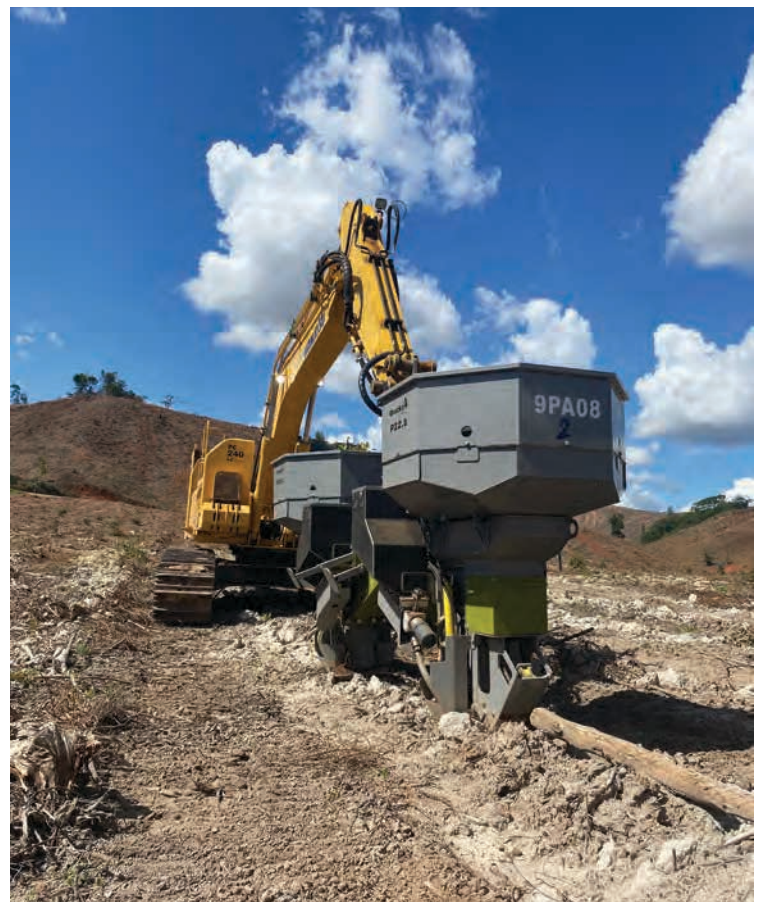
Bracke P22.b is mounted with a rotator and link that allows seedlings getting planted in a upright position.
