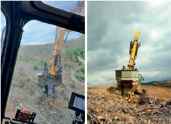
Bracke PI 2.b has a side tilt function that allows seedlings getting planted in a upright position when working in slopes.
