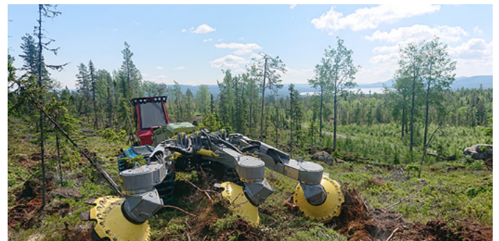
The Bracke T35.b is suitable for large scarification jobs and attaches to large prime movers.
