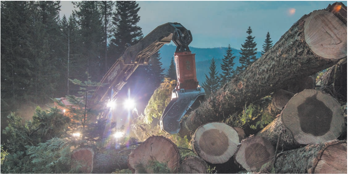
Danielson Logging has an assortment of Quadco forestry attachments, including the Quadco brand, Southstar, and Log Max. Above, a TimberPro TL765C machine is shown working with a Southstar FD750 felling head.
